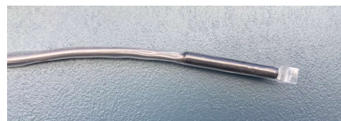
Figure 12. Temperature sensor inside heat shrink tube
